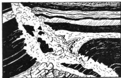
FIGURE 8.— Displacement of Coal Bed by Clay-vein. One-seventieth natural size.
